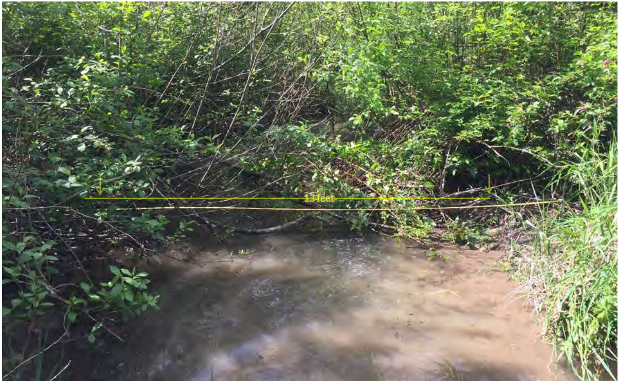
Figure 2. Cross-section #2 is influenced by beaver activity but in a transitional reach between the entrenched channel downstream and the unconfined channel condition upstream.
